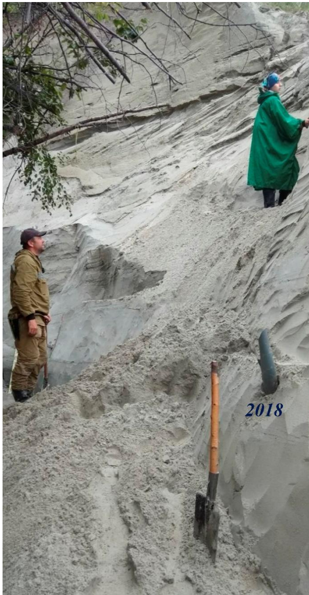
Figure 4. Obtaining the data for geological cross-section of the “diagonal sands” in the outcrops of the right bank of the River Ob’ upstream of the Settlement Khashgort (locality Bolshaya Ob’) and the pieces of PVC pipes buried during a riverbank collapse incident in 2018
